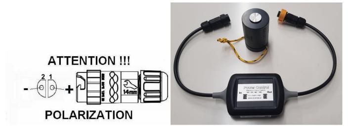
Note: When connecting a battery other than the Smart-Tex, pay attention to the correct polarity on IN as photo
